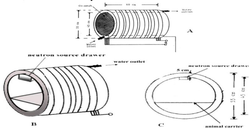
**Figure (1):** Irradiation facility for mixed neutron and magnetic fields (A) show the solenoid, (B and C) show cross section at the mid of the solenoid showing the position of  $^{252}\text{Cf}$  source.
