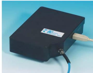
**Figure 2:** Shows the spectroradiometer to measure Color Temperature (CCT) and Color Rendering Index (CRI) for these lamps.
