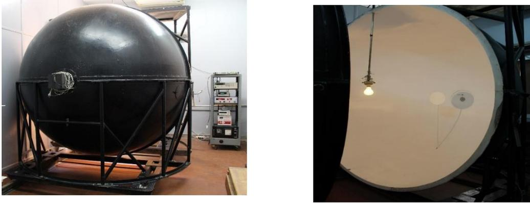
**Figure1:** The integrating sphere system.
