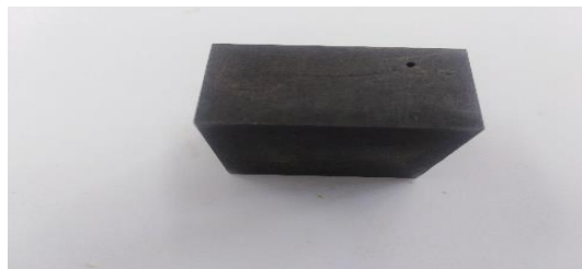
Figure 2. Steel specimen with FBH at about 9 mm from the specimen's surface.
