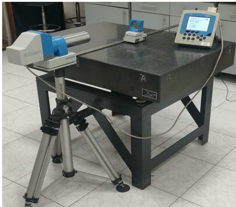
Figure 2: Flatness measurements by autocollimator system
