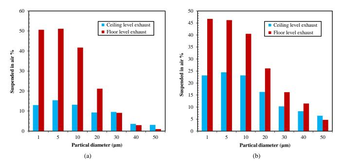
**Figure 7:** Relation between particle diameters and particles suspended in the air with different exhaled velocities (a) Exhaled velocity 0.12 m/s, (b) Exhaled velocity 2 m/s [54].
