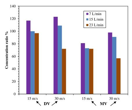
Figure 8: Comparison between mixed and displacement ventilation with different breathing rates [54].
