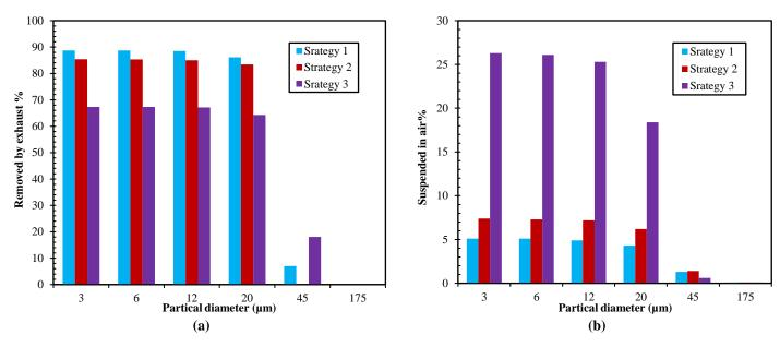
Strategy 1: Inlet and outlet are on the same sidewallStrategy 2: Inlet and the outlet are on the opposite sidewallsStrategy 3: Inlet mounted on the ceiling and two outlets are installed on the sidewall opposite of the entrance door
