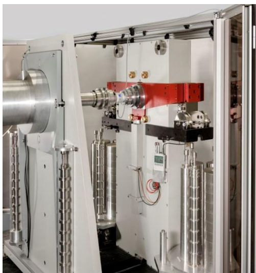
Figure 2: Photograph of 1 kN·m torque calibration machine on the left (PTB) and its main components on the right.
